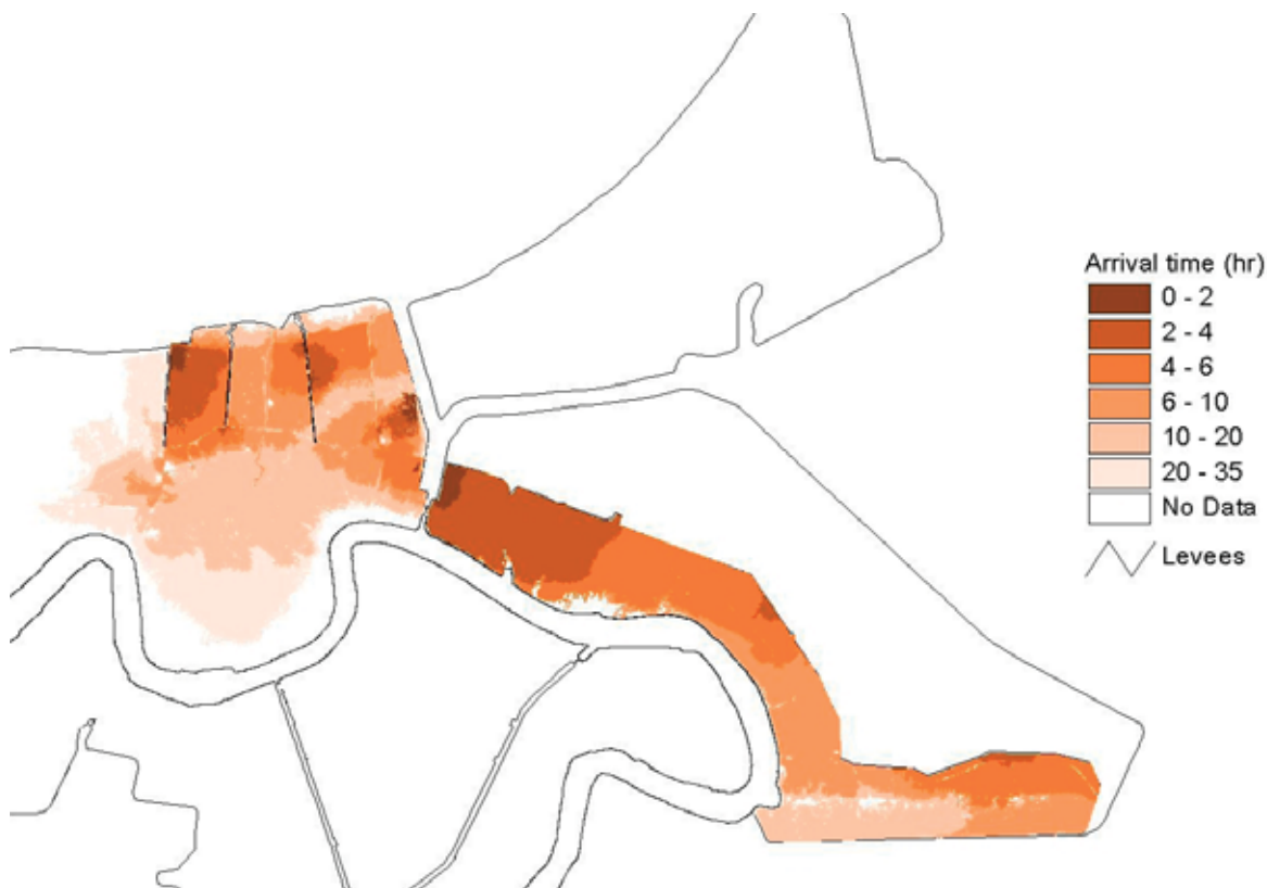
Figure 8-9: Simulated arrival time of the water for the Orleans and St. Bernard bowls after the initial breaches.
