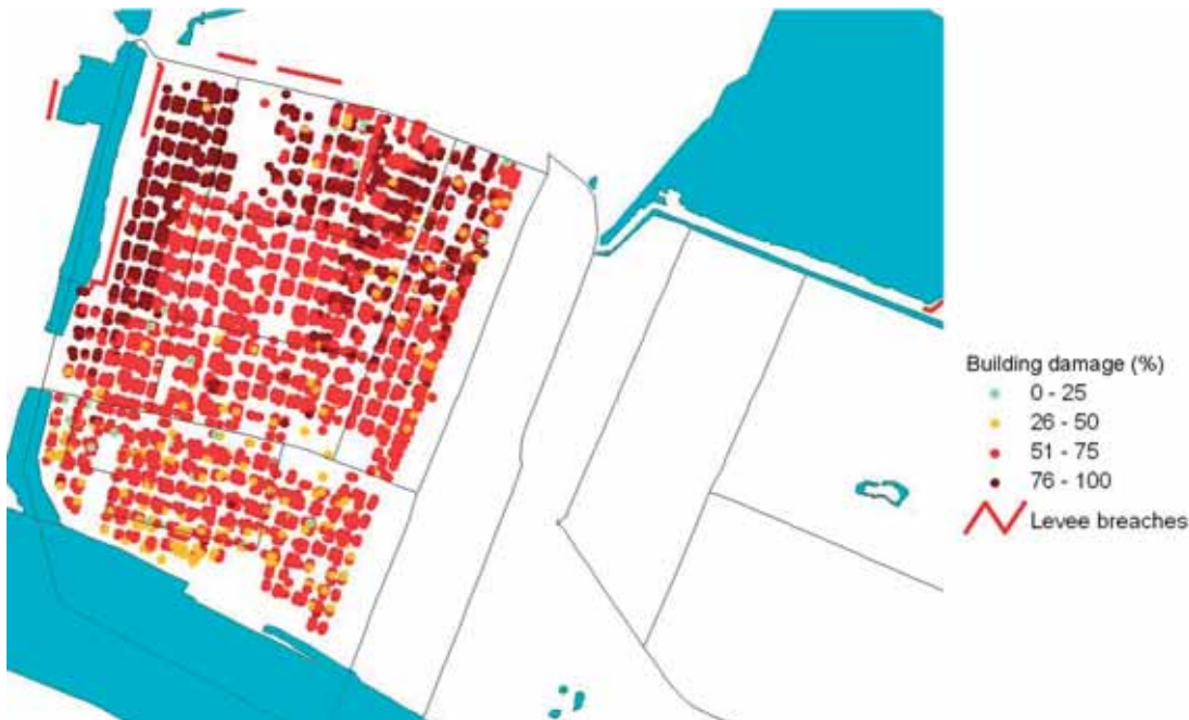
Figure 8-18: Building damage in the Lower 9 th Ward (source: http://www.unifiedneworleansplan.com/home2/section/24 , accessed December 2006. Damage levels determined in FEMA's post Katrina damage assessments. Note: scale differs from figure 8-17).
