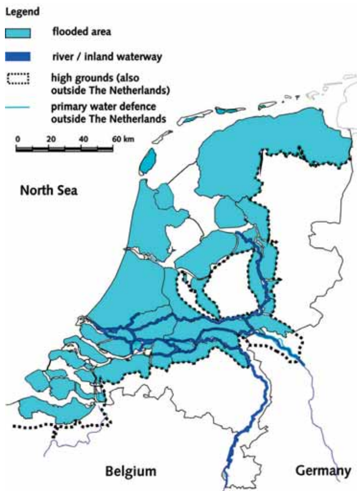
Figure 7-1: Parts of the Netherlands that could be flooded without flood defences (Source: Rijkswaterstaat)
