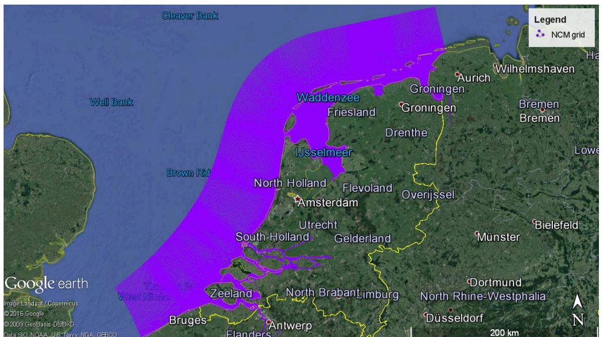
Figure 5.15 Netherlands Coastal Model grid.
