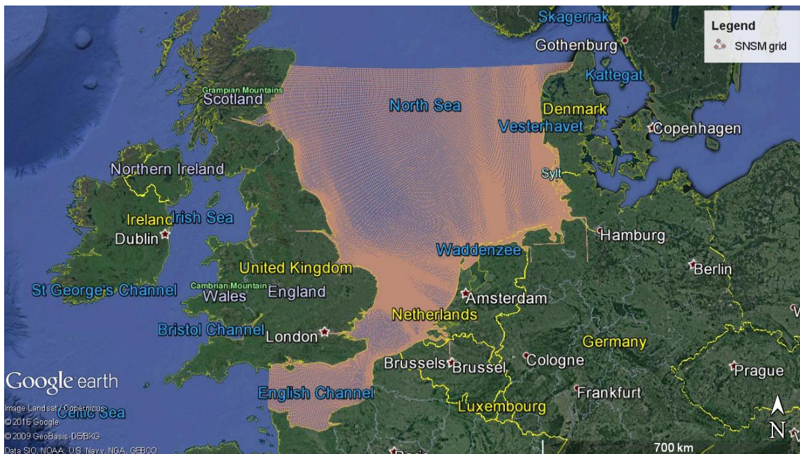
Figure 5.9 Southern North Sea Model grid
