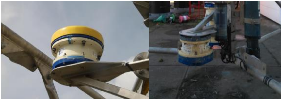
Figure 3.1 Upward-looking ADCP used on each campaign (left), downward-looking ADCP (right) used on Frame 4 during the DV campaigns.
