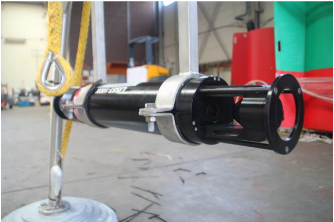
Figure 3.12 LISST-100X installed on Frame 3. The sensor is visible in the circular opening on the right side of the instrument.
